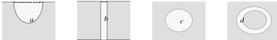
Figure 11. Holes come in superficial hollows ( a ), perforating tunnels ( b ), internal cavities ( c ), and some mixed cases, e.g. internal tunnel-cavities ( d ).
