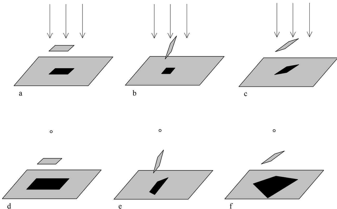
A square caster casts its shadow onto a screen. Left column, plane of the caster parallel to the plane of the screen; middle column, square tilted with two sides of the square parallel to plane of screen; right column, square tilted with no sides of the square parallel to plane of screen. Top row, source at infinity; bottom row, source close. Projection of the shadow is metric (a), affine (b-c), similar (d), projective (d-e).
